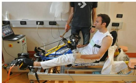
**Figure 3. An adjustable recumbent sport handbike, which is converted into an ergometer**
